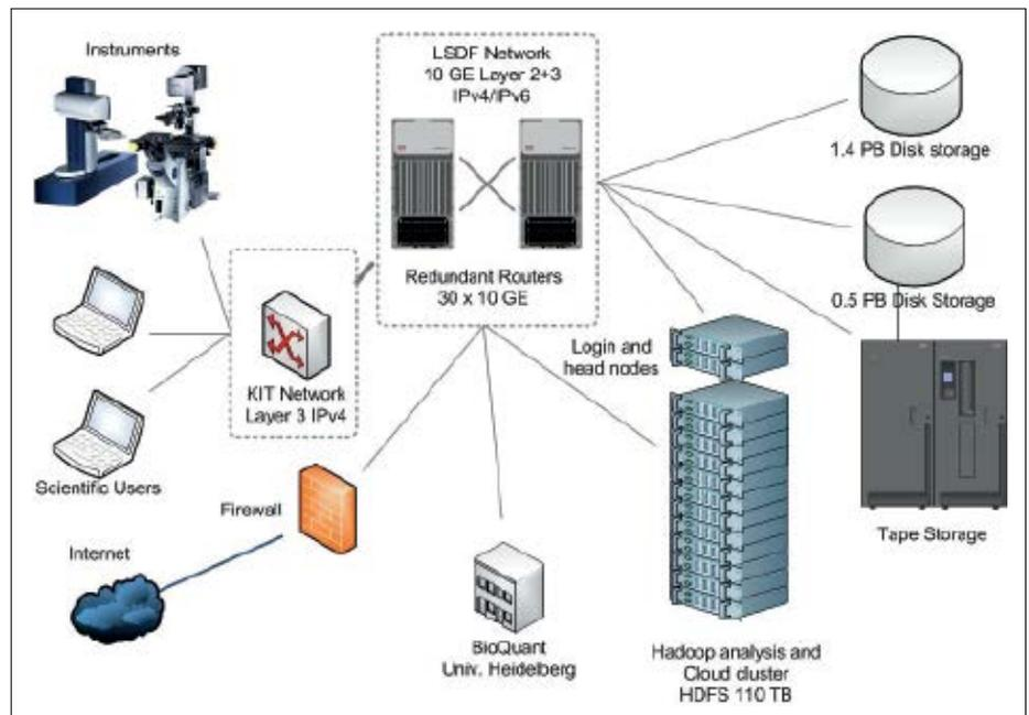
Fig. 2: The LSDF at KIT tightly integrates massive storage and archives with online computing.
